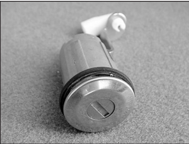
32. With the tailgate lock removed
